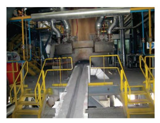
Figure 3. Photograph of a turn-key cupola furnace (EC&S, 2019). The large cylindrical structure above the base is the cupola with tuyeres on its sides. Refined metal flows from the archway at the base down the ramp.
